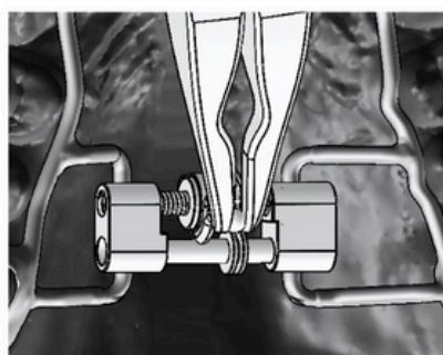
On the way down, ensure that the two gears do not engage
